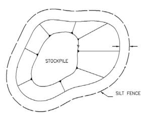
Ensure there is a buffer between the stockpile and the silt fence. Small stockpiles (less than 20 feet in diameter) should have at least a 3-foot buffer between the edge of the pile and the silt fence. Large stock piles (greater than 20 feet in diameter) should have at least a 10-foot buffer between the edge of the pile and the silt fence. Ideally, there should be a vegetated buffer beyond the silt fence to intercept suspended particles that may flow through the silt fence barrier.
