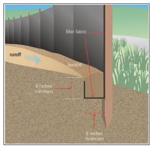
Install silt fence prior to land disturbing activities. Silt fencing should be installed 6 inches deep, at a minimum. Make sure wooden stakes are on the downstream side of the flow.
