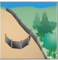
Install "J-hooks" along extended portions of diversion silt fence to promote ponding and minimize the potential for silt fence failure.
