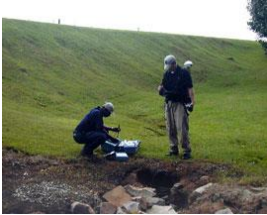
Example of field crew collecting GPS data and conducting dry weather screening protocols. Stormwater Magazine. January 2004.
