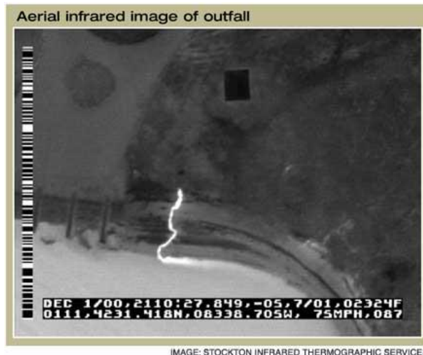
Example of illicit discharge identified via infrared aerial photography. Stormwater Magazine. March 2004.
