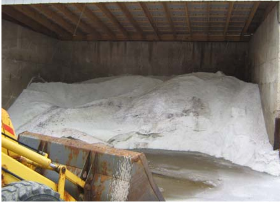
Storing rock salt in a covered dome helps to protect surface and ground water from chloride contamination.
